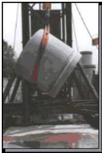
Figure 4: View of a drop test (1.2 m)
