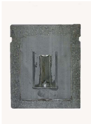
Figure 2: Section of a 1.23 m 3 concrete container with a RCV [CVCS] cartridge inside
