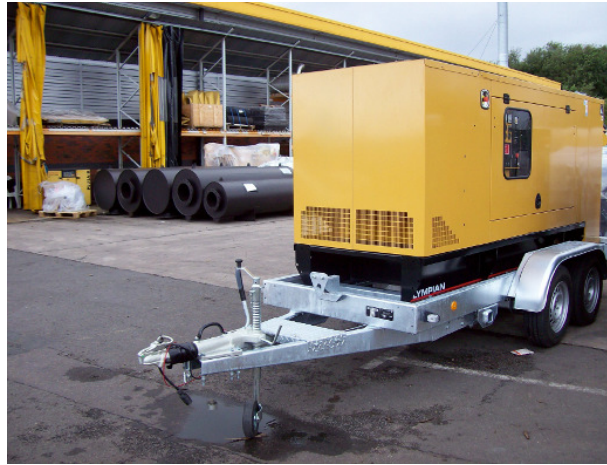
Trailer Mounted 180kVA diesel generator
