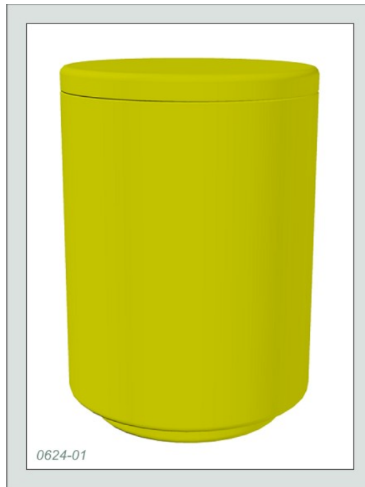
Figure 6 Illustration of a cast-iron cask as proposed for packaging of operational ILW in the EPR Variant Case 2
