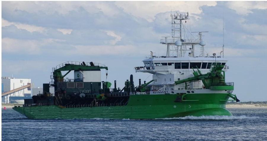
Graphic 3.2 Example of a trailer suction hopper dredger
