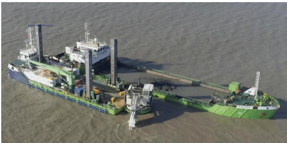
Graphic 3.1 Example of a backhoe dredger and supporting split hopper barge
