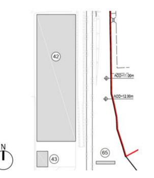
Figure 2–5: Location of the Hinkley Point Substation (65) in relation to the ISFS (42) and new Equipment Storage Building (43) from Site Layout Plan (drawing reference HINK-A1-SL-00-GA-010) in PEIR Plans - Proposed Changes On-Site
