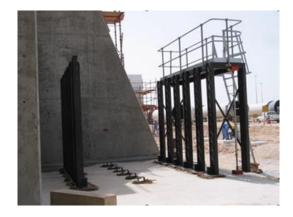
Figure 2–7: Example of a toaster-style storage rack from Flamanville 3
