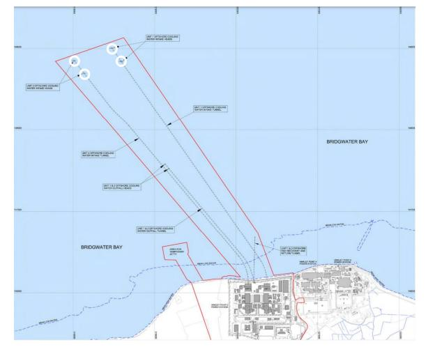
Figure 2–1: Locations of the four cooling water intake heads at which AFD systems were proposed to be installed (indicated by four white circles)
