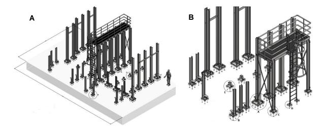
Plate 2–1: Toaster-style storage rack (A: Large rack; B: Small rack)
