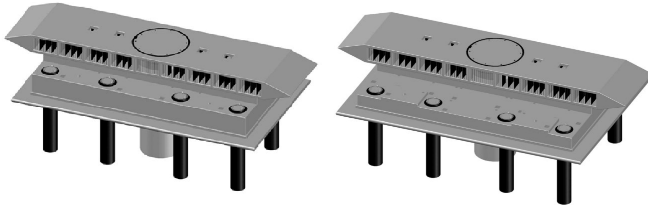
Plan 2: 3 Dimensional views of the intake heads (Type 1 on the left and Type 2 on the right; only the foundations are different; hydraulic performance are the same for both types)
