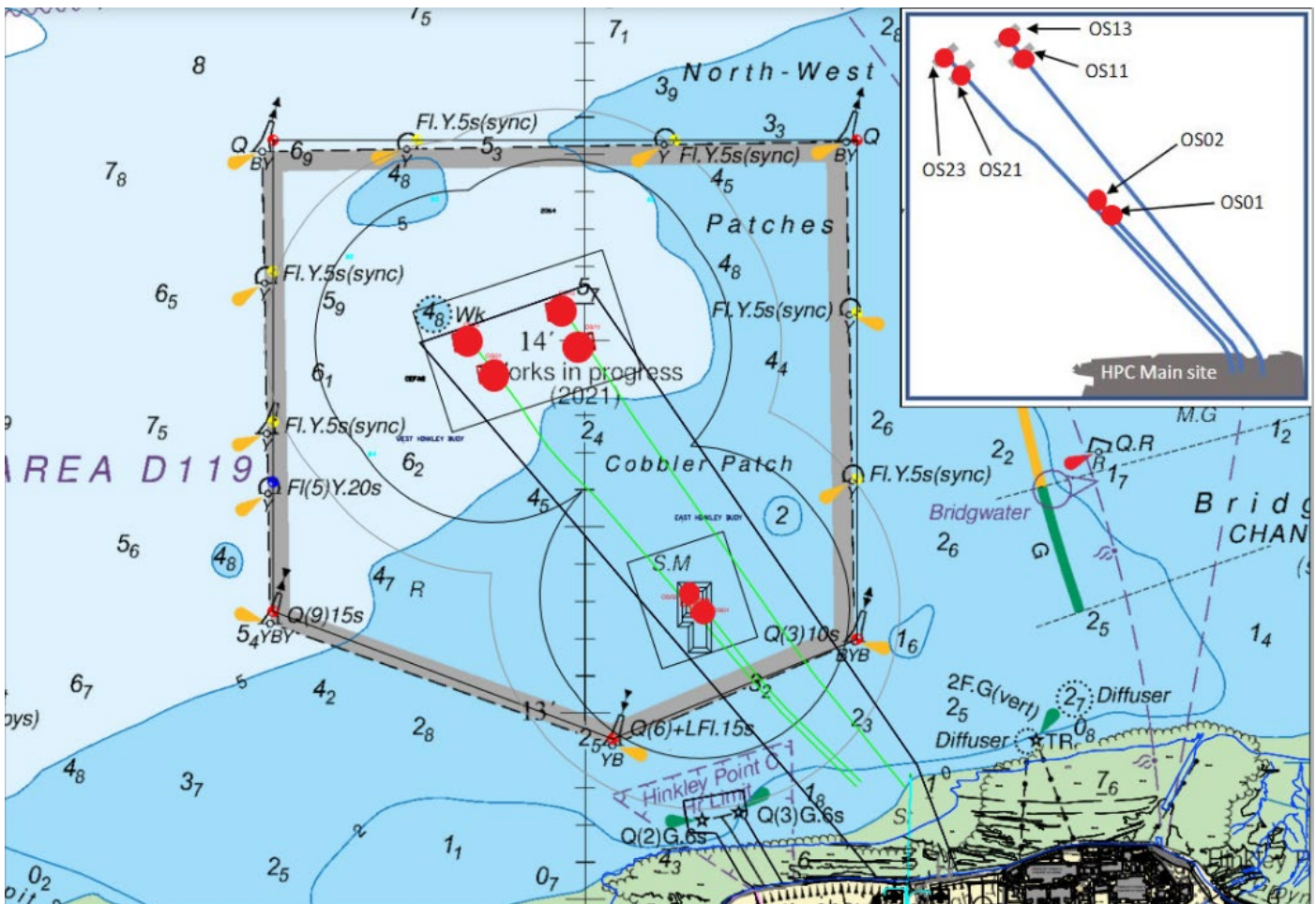
Chart extract of the HPC 'works in progress' marine construction area highlighting (in red) underwater obstructions.
