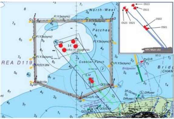
Chart extract of HPC marine works in progress area and identification of HAF structure locations (red dots).
