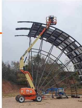
Drum Screens – manufacturing in progress.
