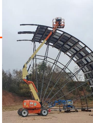
Drum Screens – manufacturing in progress.
