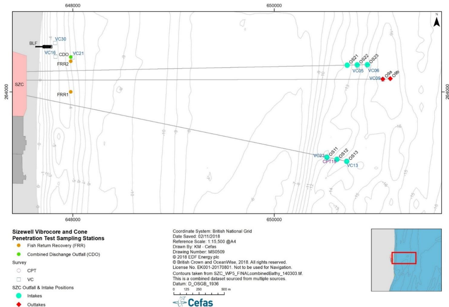
Figure 59: Geotechnical survey locations using vibrocores (VC) and cone penetrometer testing (CPT) (Fugro, 2015). Note that there are only two intake heads at each site – three are shown as the final locations have yet to be selected. 2019 geotechnical survey results are not yet available for reporting.
