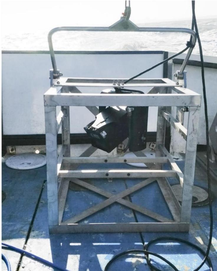
Figure 1: Frame and acoustic imaging camera setup used in field surveys. Frame is lowered to seabed and the camera rotated 360° and tilted up or downwards remotely by survey crew aboard the vessel.
