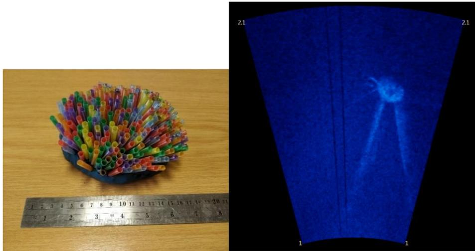
Figure 4: Section of model reef used to ground truth acoustic image footage and measurements (left) and *in situ* footage of the model recorded using the acoustic imaging camera (right).
