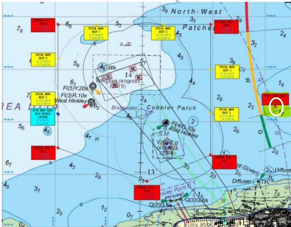
Chart extract of HPCCHA buoyage and identification of port hand later mark (white circle).
